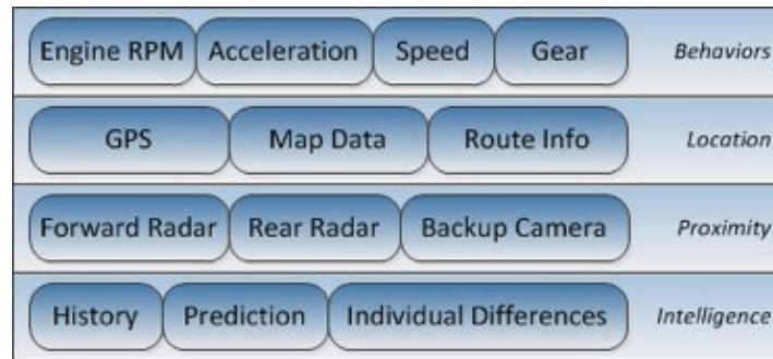
Figure 30: Functional layers of a theoretical sudden UA mitigation system
